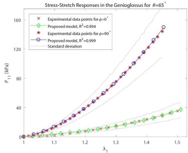
Fig. 5. Stress-stretch responses of the bovine genioglossus muscle tissue to the uniaxial tension tests in different loading angles with respect to the MF direction. Also, the best approximation of the proposed model is plotted.
