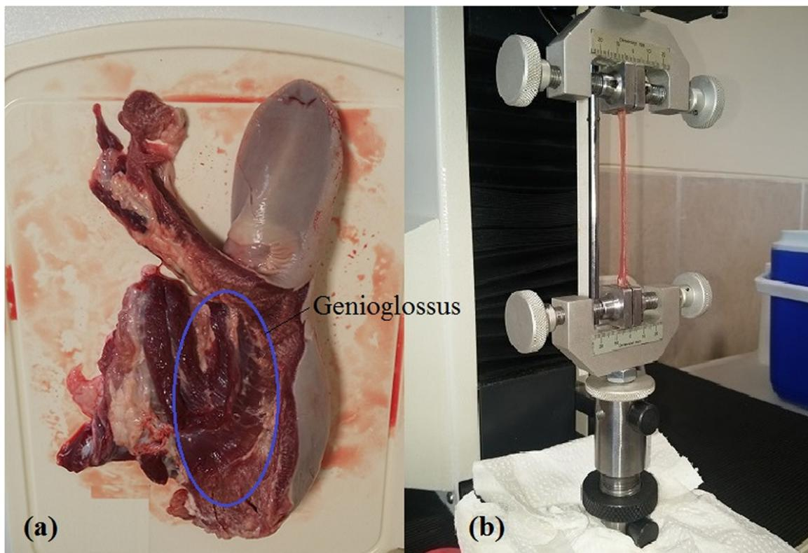
Fig. 4. Bovine tongue (a) and a sample of bovine tongue muscle under uniaxial tension test (b).
