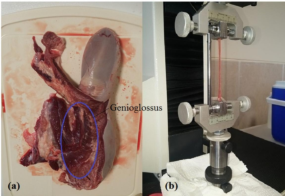
Fig. 4. Bovine tongue (a) and a sample of bovine tongue muscle under uniaxial tension test (b).
