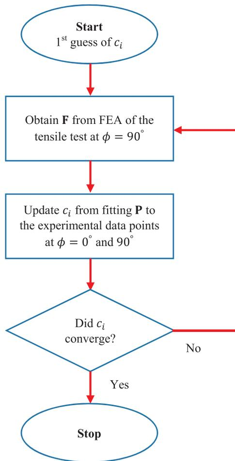
Fig. 3. Flowchart of the material parameters estimation procedure for muscle tissue via uniaxial tensile tests.
