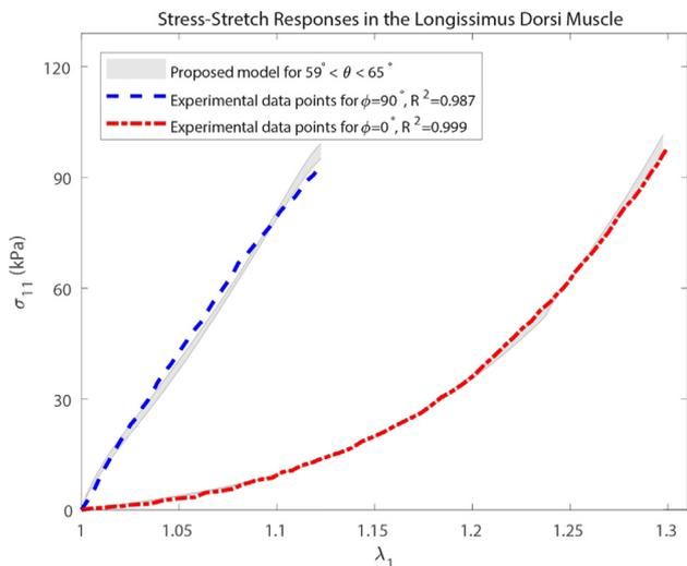
**Fig. 9.** Stress-stretch responses of the pig longissimus dorsi muscle tissue to the uniaxial tension tests in different loading angles with respect to the fiber direction. Also, the ranges of the best approximations of the proposed model for  $\phi = 0^\circ$  and  $90^\circ$  are depicted as gray bands.
