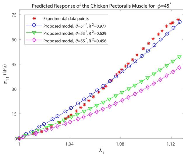
Fig. 12. Comparison of the accuracy of the stress-stretch prediction of the proposed CL for the chicken pectoralis muscle tissue in loading at different angles  $\theta$ .
