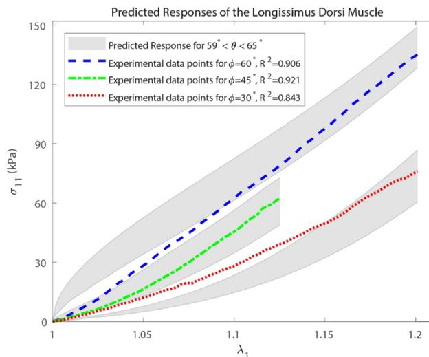
**Fig. 10.** Comparison of the accuracy of the stress-stretch prediction of the proposed CL for the pig longissimus dorsi muscle tissue in loading at different angles  $\theta$ .
