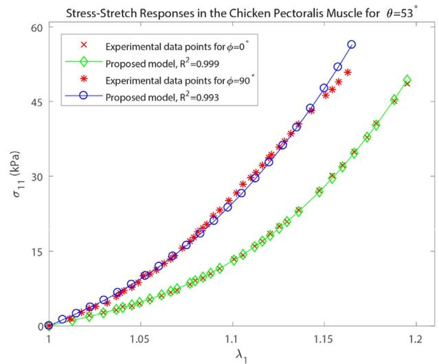
**Fig. 11.** Stress-stretch responses of the chicken pectoralis muscle tissue to the uniaxial tension tests in different loading angles with respect to the MF direction. Also, the best approximation of the proposed model is plotted.
