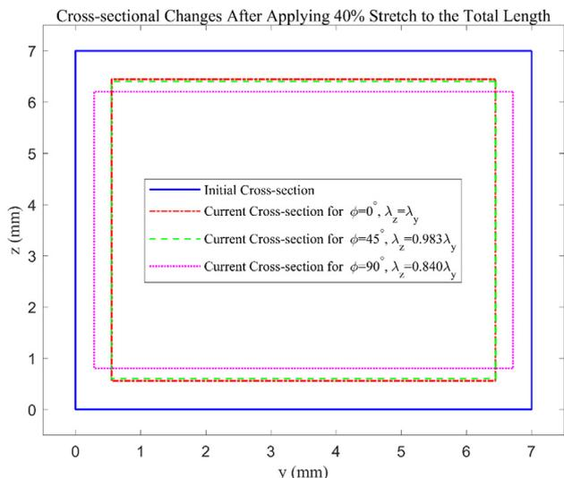
**Fig. 8.** Changes in the middle cross-section after applying 40% increase to the total length (x-direction) in the genioglossus muscle. In the case of  $\phi = 0^\circ$ , there is a symmetric deformation in the transversal directions y and z. In the case of  $\phi = 45^\circ$  in which the MFs are in the plane xz, the amount of shear deformation is a parameter that affects the values of the transversal stretches. Also, for  $\phi = 90^\circ$ , the MFs are along the z-direction.
