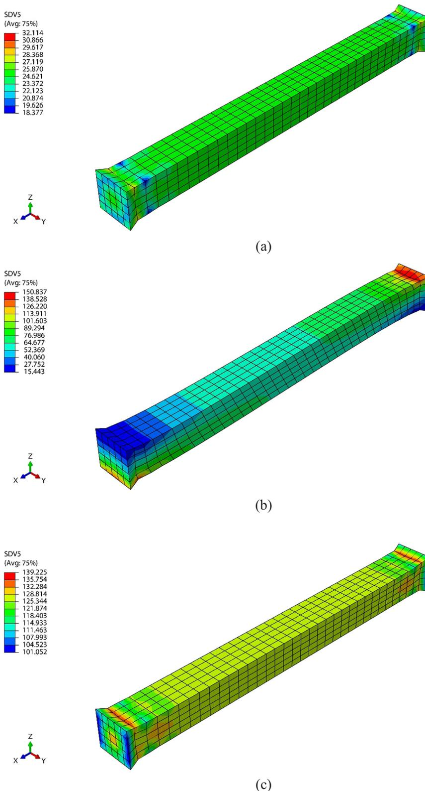
Fig. 7. Distribution of the nominal stress  $P_{11}$  after applying 40% of stretch to the total length in the genioglossus muscle for  $\theta = 63^\circ$ . (a) is for  $\phi = 0^\circ$  and MFs are along the x-direction, in (b) the direction of MFs makes angle  $\phi = 45^\circ$  with the x-direction in the plane xz, and in (c) MFs are along the z-direction which means  $\phi = 90^\circ$ .
