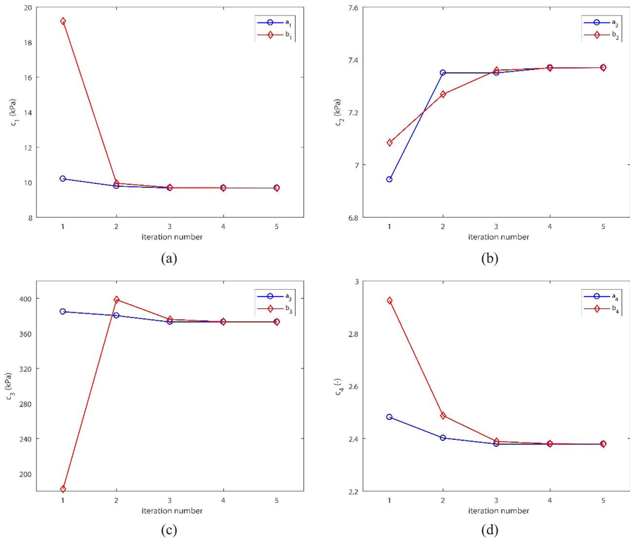
**Fig. A1.** Convergence study of the material parameters for the case of  $\theta = 60^\circ$  using two different sets of initial values, graphs (a)–(d) show changes in  $c_1$ – $c_4$  in each iteration, respectively.
