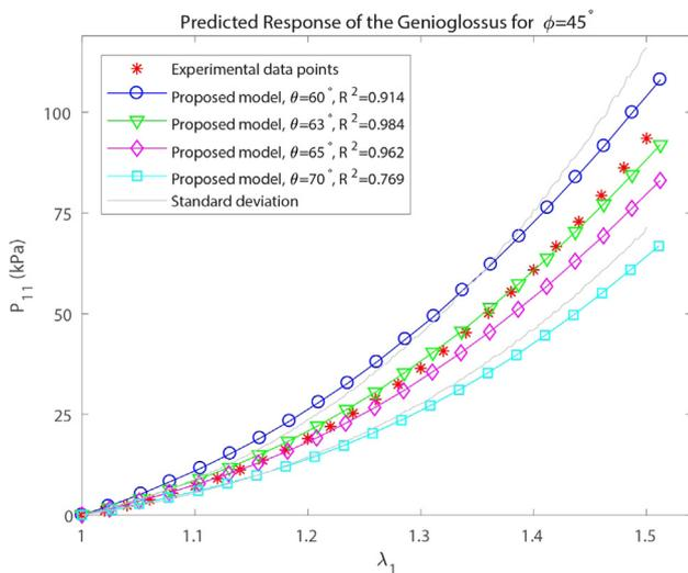
Fig. 6. Comparison of the accuracy of the stress-stretch prediction of the proposed model for the bovine genioglossus muscle tissue in loading at different angles  $\theta$ .
