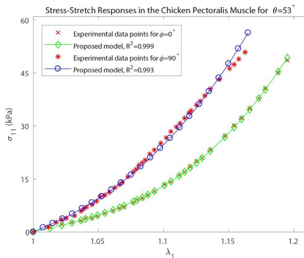
**Fig. 11.** Stress-stretch responses of the chicken pectoralis muscle tissue to the uniaxial tension tests in different loading angles with respect to the MF direction. Also, the best approximation of the proposed model is plotted.
